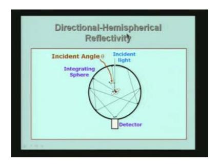
We have already seen what happens at a surface, when reflection takes place for an arbitrary surface. So the radiation is going to leave in all directions, and now I am going to integrate the radiation leaving. In the previous case the radiation incident on the surface was integrated but in this case we are integrating the reflected radiation. Therefore it is incident at a given angle and then reflected along all the
