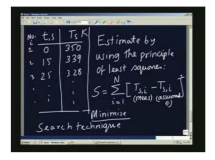
So how do we get the emissivity from such a curve?
