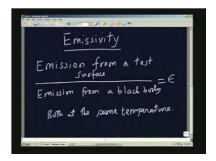
We remember the idea of brightness temperature. It was defined in such a way that epsilon times sigma times  $(T_B)$  whole power 4 where  $T_B$  is the brightness temperature of the object, is equal to epsilon sigma  $T_{\text{actual}}$  to the power of four when I am talking about total parametry that means I am using the entire spectrum of radiation.
