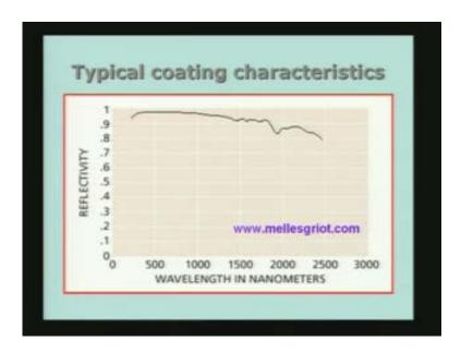
So this is the typical coating. This is the patented coating which they use in the manufacturing process. Let us now look at the apparatus known as the integrating radiometer. This is slightly different from what we have discussed earlier. In the earlier case, the integrating sphere was actually coated with a diffused surface or
