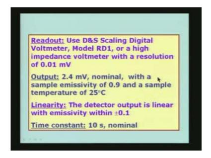
The output is 2.4 millivolts nominal with a sample emissivity of 0.9. That means if you use the high emissivity sample the output of the instrument is 2.4 millivolts and a sample temperature of 25 degree Celsius as we have taken in this particular case.
