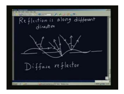
Therefore even though parallel radiation is falling on it this is going in this direction, this is going in this direction, this is going in this direction therefore you see that the reflected radiation is going in all sorts of directions. So reflected direction is along different directions. In principle, if we define a surface being totally rough engineering-wise, then what it means is that the radiation which is
