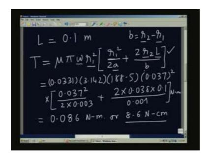
So in the case of a viscometer having linseed oil in the gap it requires about 16.2W or so much of power is dissipated because of the friction because of the viscosity of the fluid and I am rotating it at 800 rpm.
