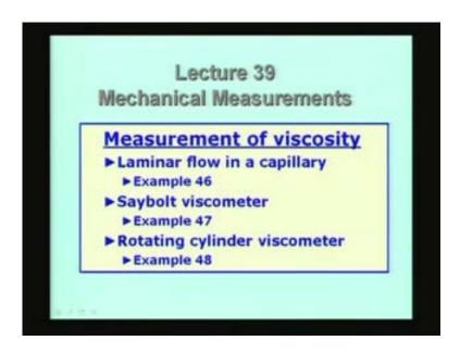
The first one will be use of laminar flow in a capillary tube which can be used for both liquids as well as gases. The second one is the Saybolt viscometer which is useful only for liquids and rotating cylinder viscometer which again is used for liquids. We will try to understand the underlying principles as well as present examples to get ideas as to the kind of numbers which are involved in such operators.
