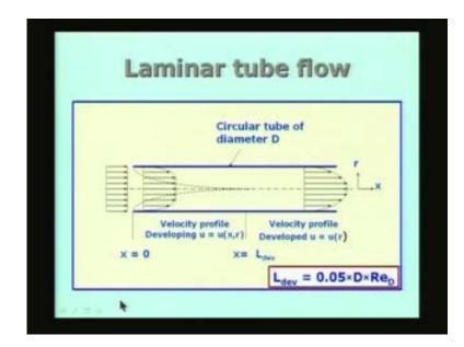
The laminar flow in a tube is taken as the model for the first method. Before we take a close look at the laminar tube flow, let us just digress a little bit, and understand what viscosity is just to get an idea as to what we are talking about. Viscosity is the property just like thermal conductivity. Thermal conductivity actually comes into picture, when heat is conducted or in the presence of a temperature field or temperature gradient.
