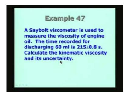
This is Example 47: I have used a Saybolt viscometer, it is used measure the viscosity of engine oil, engine oil is used in applications like IC engines and so on
