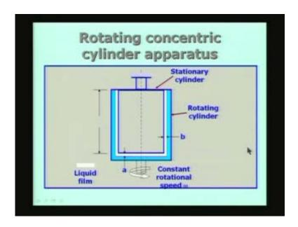
The apparatus actually consists of a stator, or stationary cylinder, which is supported here. This is a support so this is a stationary cylinder and there is a rotating cylinder. And between the stationary cylinder and rotating cylinder there is a small gap b, of course, at the bottom also there is a small gap a and this outer
