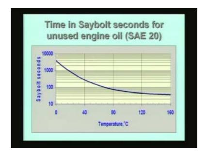
What I have done is, to make a simple plot showing what would happen if I were to use SAE 20 unused engine oil. It is a lubricant of relatively low viscosity SAE 20 and all I have done is taken the data for engine oil which is in the form of temperature versus viscosity of kinematic viscosity and I have used it in Saybolt viscometer by using a thought experiment, and I want to find out what will be the drainage time which is measured in the experiment if it were performed. So if I
