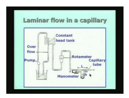
So what we will do is we will assume that somehow we are able to maintain the velocity to a value such that for a given fluid whose viscosity we want to measure using this apparatus the Reynolds number is less than the critical value. If it is not less than the critical value we will have to adjust the flow rate such that it comes below the critical value. So, what is required for the apparatus is very simple. I require a certain length of tube, I have to allow for developmental length and the
