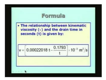
The kinematic viscosity nu is given, as a function of the time for drainage of 60 mm of the liquid through the viscometer so [0.00022018 t minus 0.1793 by t] into 10 to the power minus 3 m square by s, this is the unit. So the kinematic viscosity is a function of the time for drainage. Let us look at a typical example.
