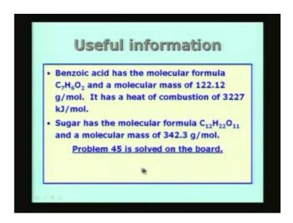
Benzoic acid has a molecular formula given by  $C_7$   $H_6$   $O_2$  and molecular mass of 122.12 g by mol and it has a heat of combustion of 3227 kilo joules by mol, this is known from literature. This is supposed to be accurately known. The case of sugar that I am going to burn with the second experiment has a molecular formula  $C_{12}$   $H_{22}$   $O_{11}$  and a molecular mass of 342.3 g by mol, this will be useful for solving the problem.
