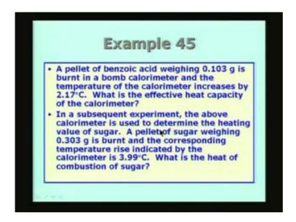
So what is the effective heat capacity of the calorimeter? It is determined from this part. In a subsequent experiment the above calorimeter is used to determine the heating value of sugar. A pallet of sugar weighing 0.303 g is burnt and the corresponding temperature raise indicated by the calorimeter is 3.99 degree Celsius, what is the heat of the combustion of sugar? These are the two parts of the problem. Now let us look at some of the useful data or useful information.
