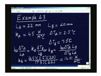
The temperature difference is the same. When you represent temperature difference it can be either Kelvin or degree Celsius. And we also have measured  $deltaT_B$  of the second material, as 7.3 Kelvin or degree Celsius. So all I have to do is to use the simple rule,  $k_A$  delta  $T_A$  by  $L_A$  is equal to  $k_B$  delta  $T_B$  by  $L_B$  or  $k_B$  is equal to  $k_A$  delta  $T_A$  by delta  $T_B$  by delta
