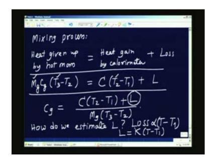
This is the equation, I am measuring  $T_2$ , I am measuring  $T_3$ , I know mass of the solid which is transferred, I can actually use this expression to determine  $C_g$  which is nothing but C into  $T_2$  minus  $T_1$  plus L by  $m_g$  into  $T_3$  minus  $T_2$ . So this is the problem, all these are measured in this, so how do we estimate L?
