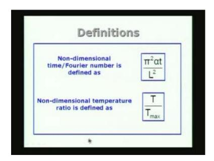
Therefore you take y square alpha t which is measured divided by 1 square is equal to 1.37 and from this I will determine the alpha of the material. The alpha is equal to 1.37 is equal to  $\pi$  square alpha t which is measured divided by 1 square, so I can determine the thermal diffusivity. The method is some what expensive ,and that is the only major drawback of the method because the laser and the temperature recorder and so on are expensive equipments.
