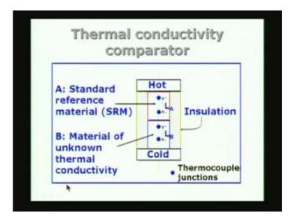
It is very useful when you have the sample available in the form of rods that is cylindrical specimens are available and if you have the Standard Reference Material
