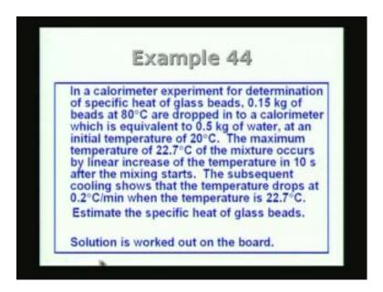
In this experiment, there is the mixing process which means mixing in the thermal sense. Hot sample is dropped into the calorimeter. So the temperature of the mass which is dropped is higher than the temperature of the medium either oil or water taken inside the calorimeter. Therefore the temperature of water will increase. We
