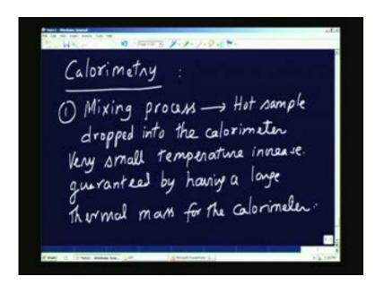
Therefore the estimation of the losses becomes the major problem so you may you have a mixing process which consist of a hot sample which dropped in to the calorimeter, the calorimeter has got the thermal mass which much larger than thermal mass of the material which is being dumped in to it The second part consists of a cooling process. In this sketch here this is the time axis, this is temperature. I have the calorimeter at temperature  $T_1$  which is also the temperature
