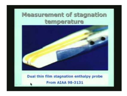
In this case you can see the body is in the form of a bluff body, and at the front stagnation probe two film gages are placed close to each other. Now we heat these two films to different temperatures to start with. By passing a current or by placing a heater just behind the thin film gages we bring the temperature to two different values.
