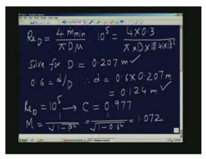
So, I use equation 6 of course, with the assumption that Y equal to 1. There is no expansion factor, the compressibility effect is not there. Therefore I can say delta p minimum by using that
