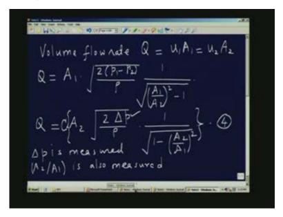
When writing the equation I wrote down the pressure as  $p_1$  here, and I also wrote the pressure as  $p_2$  here. The question is, what we are going to do in practice is to measure the pressure at the wall and here, we are going to measure  $p_2$  at the wall. If there is some viscous effect, the viscous
