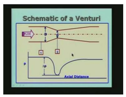
So it starts converging from D to a small diameter **d** and again it starts diverging and it goes back to the original diameter of the thing. Of course the disadvantage of venturi is that it requires a long length for the measuring device, the venturi itself is very long, from here to here is a fairly long thin, way compared to either the orifice plate which is just a small plate with a hole in it, or
