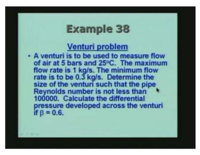
And we want to find out what is the size of the venturi such that the pipe Reynolds number is not less than 100,000. In that case you want to calculate the differential pressure developed across the venturi if the beta is point six. This is example 38.
