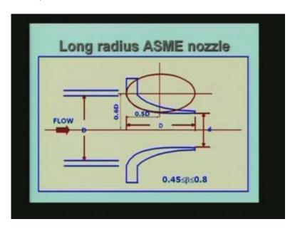
This is the nozzle as shown here, exit diameter is d, inlet diameter is d here and the nozzle itself is controlled as the part of the ellipse, from here to here is part of ellipse and the major axis equal to d is the diameter d displaying this d and the semi major axis will be 0.6d minus 0.5d into 2 because that will give this. Therefore this is the standard procedure for obtaining the long radius
