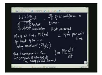
So all we have to do is equate the two. So we will see that Mc dT by dt is equal to qA or dT by dt is equal to qA by Mc and initially at t is equal to 0 we are assuming
