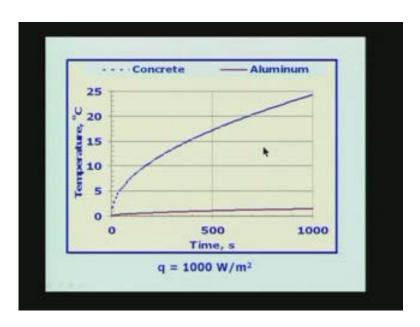
However, if we use aluminum for example, the surface temperature increase is very marginally because most of the heat is conducted into the material and therefore for the measurement of heat flux if you want a sizable temperature change I must use a material with small thermal diffusivity, small conductivity and so on. And now if I compare the response at a depth compared to the response of the surface I just have to take the ratio of the two quantities.
