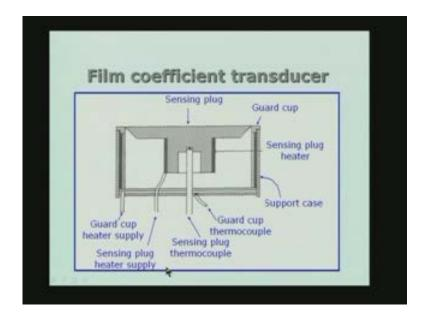
So if I want to measure the heat transfer coefficient which is a very important quantity in studies involving heat transfer especially convective heat transfer.
