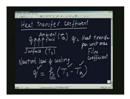
Suppose I have a surface and we have an ambient fluid which may be moving, if the surface of the temperature is  $T_s$  and the temperature of the ambient is  $T_a$  and, if I measure the heat flux at the surface, if  $T_a$  is less than  $T_s$  it will be in this direction q and q is nothing but heat transfer from per unit area, the fundamental equation is
