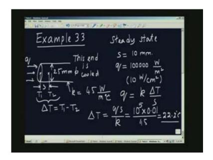
So I can find out what is delta T I am going to get, by using a simple formula q is equal to k delta T by S, the diameter of the probe does not come into the picture because we are having the heat flux and we are not measuring actual heat transfer for which of course you would require the diameter of the probe. From this I can obtain delta T as qS by k which is directly proportional to q therefore it is a linear
