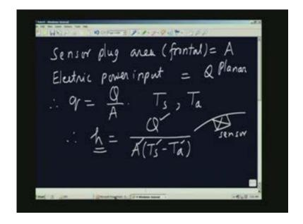
In this case I have the sensor plug surface as a planar area, so this is the planar area. And the sensor itself can be mounted on the surface and it could be placed such that if the rest of the surface is there you can make sure that you can place your sensor here. This is the surface and this is the sensor, a second arrangement is sometimes useful. It is again for the measurement of heat transfer coefficient. I use the heater in the form of a cylindrical tube.
