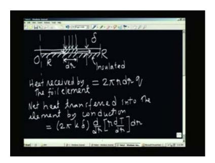
So the area is continuously changing in the radial direction. Now the heat received by the foil element must be exactly equal to the net heat transferred
