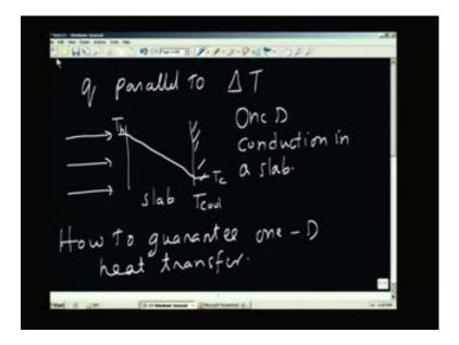
How to guarantee one dimensional heat transfer? Why is it so difficult? Suppose I have a finite size material L and this is the diameter of a block of
