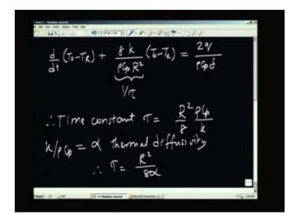
Let us take a typical example of a gage. This is example 32. It may be constructed using a 6 mm diameter foil of 50 micrometers thickness. The foil is very thin 50 micrometers and the diameter is 6 mm. The thermal conductivity of foil material is typically equal to 20 watts by m degree Celsius. So it is a copper constantan foil. So copper constantan thermocouple pair gives an output about 40 microvolts by degree Celsius.
