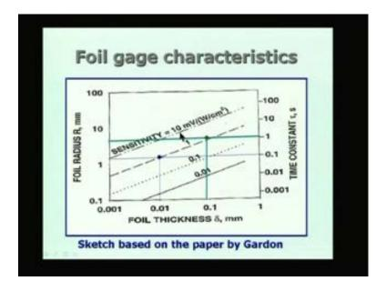
He has made a plot showing the foil thickness on the x axis the foil radius on the y axis it is a log plot and on the right hand side he has given the time constant corresponding to the R and delta values. Several lines are given here corresponding to different sensitivities. Sensitivity is nothing but the reciprocal of K so sensitivity is so many millivolts per watts per centimeter squared. This is a more usual way of representing the sensitivity.
