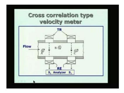
Therefore if I look at the  $S_1$  and  $S_2$ , I will get the following  $S_1$  is the signal with respect to time I get a small blip here the value of the intensity has come down because scatterer has passed through this region and I get a blip like this and after a certain time delay tau time delayed tau I get the second one which is going to show the presence of the blip.
