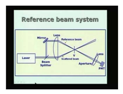
What we have is similar to the fringe system. I have got the laser, a beam splitter then the mirror so that I can create two beams of light from a single laser source, this is one beam and this is the other beam, I call this the reference beam. And in this case what I am going to do is, I am going to do
