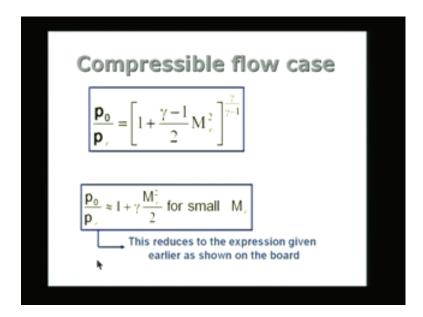
This is the piece of 0 called the stagnation pressure. We always use the 0 as the symbol subscript for stagnation pressure and  $p_{infinity}$  is the other static pressure. What does it mean? It means that when the velocity of fluid is brought to 0, how are you going to bring it to 0? If it is brought to 0 by an isentropic process then the pressure equal to the stagnation pressure indicated as p subscript 0.
