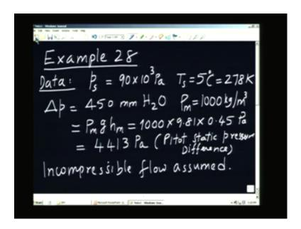
This is the pitot static pressure difference. Now I will calculate flow assumption assuming that the flow is incompressible. Of course we do not know whether it is a good approximation or good assumption but we will make the assumption first and then calculate and find out and then try to recalculate if necessary. So, if you do that let us calculate density  $\operatorname{rho}_{infinity}$ , or if you want you can call it as  $\operatorname{rho}_s$ .
