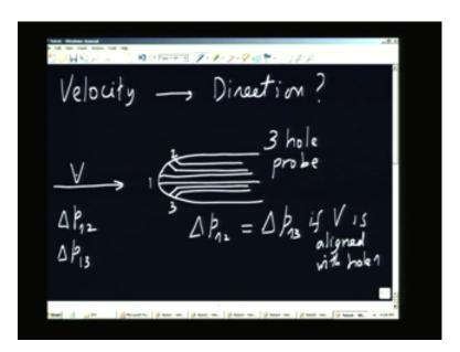
Therefore I will be able to actually use the probe and find out the velocity as well as the direction by using that kind of information. If the velocity vector is in some arbitrary direction, and the probe is oriented again in an arbitrary direction with respect to flow velocity you can in fact think in terms of a multiple hole probe one at the center.
