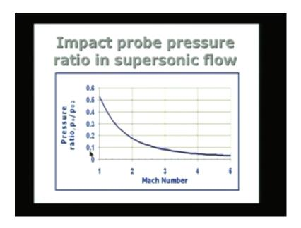
So in the impact probe I am going to measure the static pressure in the mean stream which is coming in, I am going to divide by the pressure indicated by the pitot tube so this ratio is going to be related to the Mach number of the stream. So we can use a graph of this type to measure. For the y axis whatever is indicated is measured, the x axis gives the corresponding Mach
