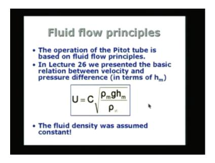
Assumption of constant density is valid strictly in the case of liquid flows. So we say that incompressible flow assumption is valid for most liquid flows. Of course when the temperature does not vary too much within the flow in medium then we can say incompressible or constant density assumption is alright. Also in the case of gases incompressible flow assumption is valid if the flow velocity U, is much smaller than the speed of sound a.
