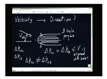
I can have a five hole probe as shown here so we have multiple holes and this can be called 1, 2, 3, 4,5. I have four different delta  $p_{s4}$  in number. So these will be depending on alpha in this direction this angle phi and you can have angle beta in that direction. That means the probe can be rotated at an angle with respect to V as shown here, it can have at an angle alpha in this plane, beta in this plane and an angle phi like that.
