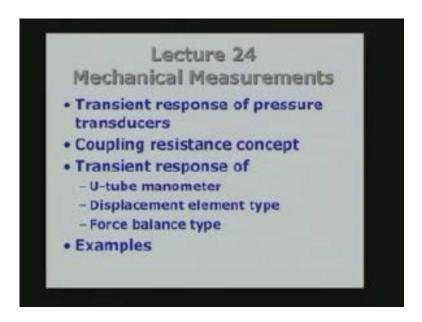
We will use the concept of coupling resistance to characterize the connection between the pressure point or the point at which pressure has to be measured and the location of a transducer. Normally the transducer is far away from the place where the pressure is being fed into it. So the resistance of the tube through which the pressure has to be propagate or the pressure information has to propagate is going to come into picture.
