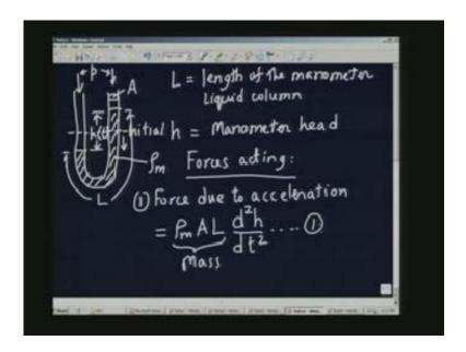
This is not the total mass, the total mass would have been  ${\rm rho_m}$  A into L which is for the entire column. Here it is only the extra height which you are having on the right side of the u-tube manometer. Then there is the viscous resistance.
