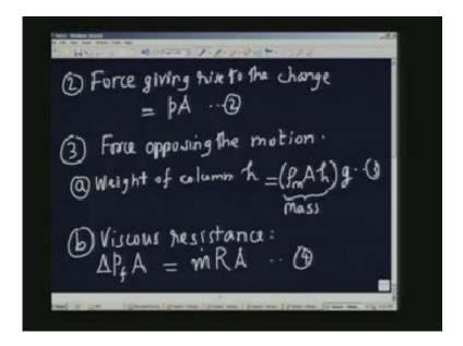
I am assuming that the entire liquid in the manometer is moving over to one side. So one would assume that each point in the liquid is moving up with a velocity equal to dh by dt, dh by dt is the velocity of the liquid and I am assuming that it is incompressible therefore the velocity is dh by dt. Now how does the viscous friction come on top of that?
