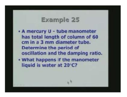
We want to determine the period of the oscillation and the damping ratio. The period of oscillation is nothing but the characteristic time and damping ratio we wanted to determine. In this case the liquid is mercury. And I also want to find out what happens if the manometer liquid is water at twenty degrees Celsius instead of mercury. If I change from mercury to water what is going to happen to the time constant and also to the damping in this particular case?
