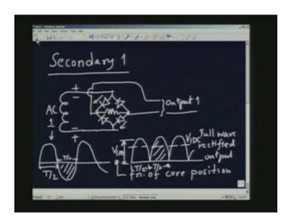
This is the full wave rectified and rectified means it is on one side only the output. And this magnitude here we will call it as  $V_{\text{maximum}}$  . $V_{\text{1m}}$  or  $V_{\text{1maximum}}$  will depend on the function of the core position. So, if the AC wave is coming here if this is positive with respect to this, this diode will conduct so the signal will pass through like that. If this becomes negative and this becomes positive the other two diodes are going to do the conduction. That
