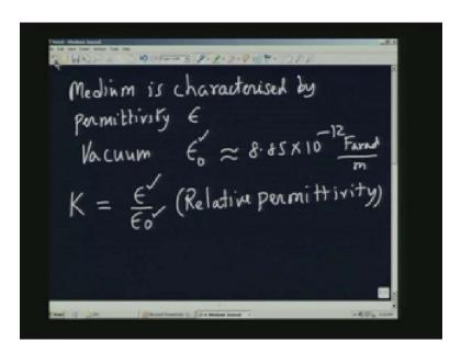
If you use a glass for example you can get about ten times the capacitance. For a given area and the distance between the two plates I can increase the capacitance by choosing the particular material which is used as a dielectric between the two electrodes. So, mica is 3 to 6. All these are mica capacitances available in the market commercially. When you want to go and buy and use it for your secured purposes you can have capacitance of mylon or mica or PVC etc.
