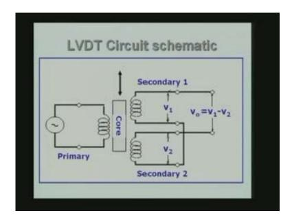
Therefore here is a LVDT and in the LVDT essentially there is a primary coil here and there are two secondary coils and there is a core which is capable of moving up and down and this is the one which moves with the pressure transducer which gives rise to a movement of the core either in the
