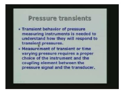
So from these reasons, it is necessary to understand how a transducer is going to behave when you have a time varying pressure applied on it. Thank you.
