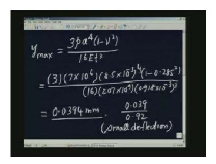
So we have a 17 mm diameter gauge almost like 1 mm thickness of diaphragm because the pressure level we are measuring is also quite large. Now let us find out what will be the central deflection.
