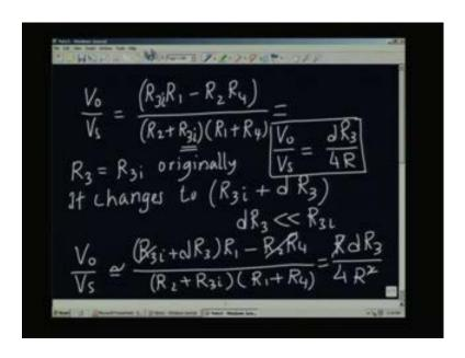
What I will do is I will say dR<sub>3</sub> by R, here R is nothing but R<sub>3i</sub>. I am writing it as R because we have made that clear earlier. This will be some S times epsilon in the axial direction where epsilon<sub>a</sub> is the strain of the element. So introducing this into the previous expression and rearranging I am going to get the following:
