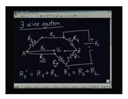
So if you look at this arm actually it is  $R_2$  plus  $R_L$ . And if you look at this arm this is  $R_3$  plus  $R_L$ . Therefore I am adding a common value of resistance to these two sides and therefore if I look at the balance equation let us see
