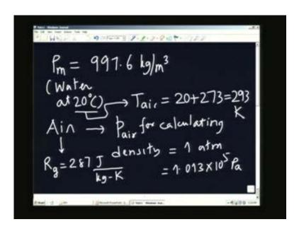
So, by using the equation of state we can calculate rho  $R_g$  times T is equal to  $p_{air}$ , from this I can calculate rho of air or the fluid in which the measurement is being made equal to p by  $R_g$  times T is 1.013 into 10 to the power of 5 by 287 that is  $R_g$  into 293 the density comes out to 1.205 kg per cubic meter.
