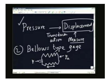
We talked about thermometers; the change in resistance is related to temperature so we measure the resistance change when we went for the temperature change. Here we are finding out what the pressure is by measuring the displacement of a diaphragm element.
