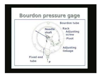
And as we have already made it clear in the previous lecture it can be used for various ranges starting from even below atmosphere to above atmosphere to very large pressures, very small pressures the Bourdon gage covers a very large range of pressure measurement. So let us look at the internal construction. The internal construction is very clear from this particular sketch.
