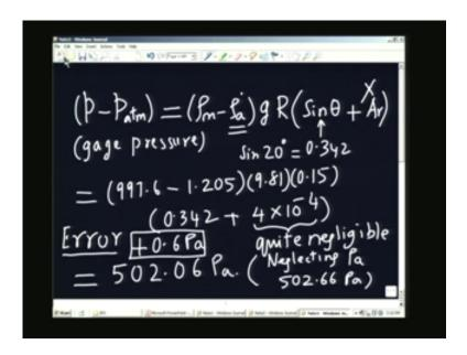
So the pressure difference if you remember will be p minus p atmosphere, what we are measuring is the difference between the pressure of the air with respect to atmosphere, this is also referred to as the gage pressure.
