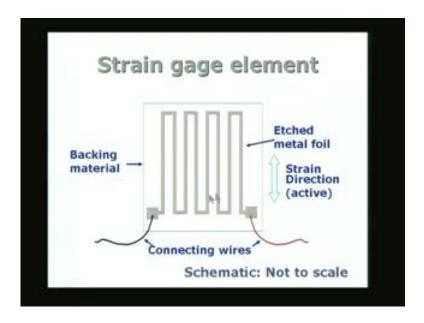
A strain gage element I said just a little while ago that we can measure the displacement using a strain gage element.
