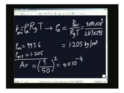
So you see that we have the water density or rho<sub>m</sub> is equal to 997.6 and the air density is 1.205 both in kilograms per cubic meter. So even in this case you can see that the difference between the densities, this density is very much higher than this, and it will be only one part in 1000 roughly or a little more than one part in 1000. So in essence, it may be alright to neglect this but of course we will take into account then we will see what is going to be error in that.
