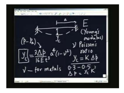
I have a displacement which is measured at the center I will call it  $y_c$  and let us take this as radius a and the material has got some mechanical properties which are going to be important.
