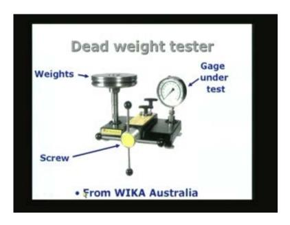
This is a dead weight tester which is commercially available and it is used for calibration purpose. Now, let us look at the other ways of measuring pressure.
