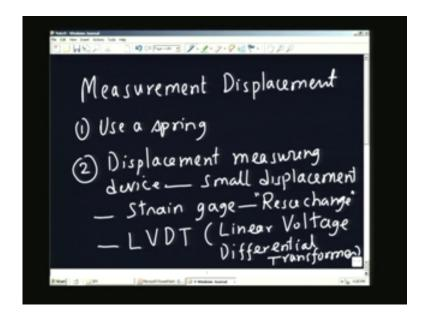
So if we are now thinking in terms of converting the pressure information to displacement information. Measuring the displacement information by using a suitable instrument or suitable transducer and then working backwards and trying to find out what the pressure is. So there are several ways of doing it. Actually we can use a spring, one is to use a spring itself.
