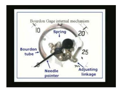
Through the sealed tube we communicate the pressure to be measured. And of course at the outside pressure is the atmospheric pressure. Or in some cases the outside pressure may be a different pressure.
