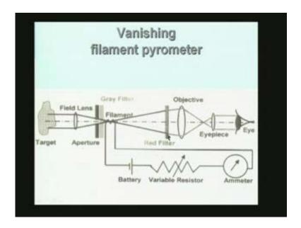
Now, to complete our discussion on the vanishing filament pyrometer, I said that we are going to choose the particular wavelength by the combination of the red filter and the eye, and that is explained in the graph here.
