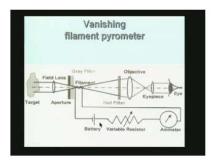
We have the target whose temperature I want to measure. I have a field lens which will gather light coming from this target, and then it will be focused on to the plane of a filament which is shown here, and the filament is actually run by a battery, a variable resistor, an ammeter and so on.
