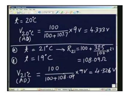
So when t is equal to 20 degrees voltage indicated by the voltage, which is, I will say that is AD, this is AD, across AD, is 100 divided by 100 plus 107.7 which is what we discussed, now determined, multiplied by this comes to 4.333. This is what happens at 20 degrees.
