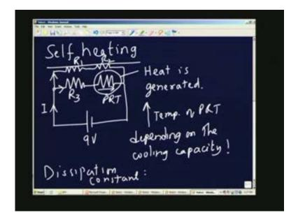
So you essentially see that there are two resistances in series across the battery. This is the PRT, RTD and this is the resistance  $R_3$ . Of course, there is one more limb in which there are other two resistances  $R_1$  and  $R_2$ , and this was 9 volts, or whatever x y some voltage. So a certain current is flowing
