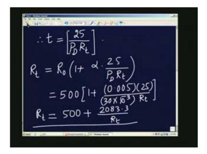
Therefore, t is actually equal to 25 divided by  $P_D$  into  $R_t$ . Suppose we make sure that all the appropriate quantities are given in the proper units so that I get the proper value for that.
