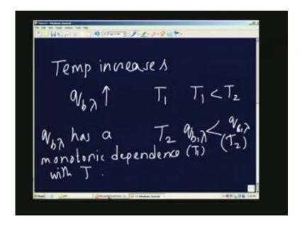
So  $q_{b\lambda}$  (T), has a monotonic dependence. Monotonic means one-sided, or one way dependence. Monotonic dependence with T. It increases if the temperature increases.  $q_{b\lambda}$  (T), also will increase. So with this, let us look at the Plancks function again.
