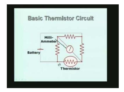
The basic Thermistor circuit I have indicated here is no different from what we had earlier in the case of a PRT. So you have a battery and you have a bridge circuit. The PRT is in one, the Thermistor is one of the limbs, and these three are fixed resistances, and what we can do is suppose we are going to use it at a particular temperature, and the vicinity of the temperature you want to measure the temperature variation.
