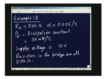
We have a PRT of 500 ohms resistance, and alpha value of 0.005 per degree Celsius, and dissipation constant is specified in this problem equal to 30 milliwatts per degree Celsius. We are also given that the supply voltage is 10 volts, and all the resistors in the bridge are 500 ohms, and suppose that the PRT is exposed to 0 degree centigrade environment, so the point to notice that is that.
