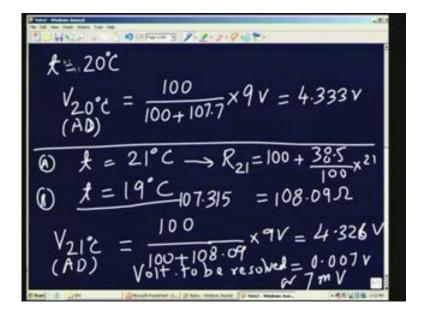
So the voltage to be resolved is the difference between this 4.333326 so that will give you 0.007 volts, or 7 millivolts. Actually, I can also calculate what
