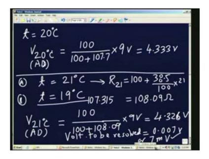
So in the case b, the temperature is 19 degrees, and the resistance at 19 works out to be 107.315 ohm, and the value of voltage across C D works out to be 4.341mV. And if you go back and check the resolution required, 4.333 and 341, so that 4.333 minus 4.341 is about 8 millivolts.
