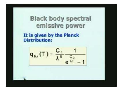
You see that the Plancks function tells me that  $q_{b\lambda}$  (T), at any temperature T is given by  $C_1$  by lambda to the power of 5.  $C_1$  is called the first radiation
