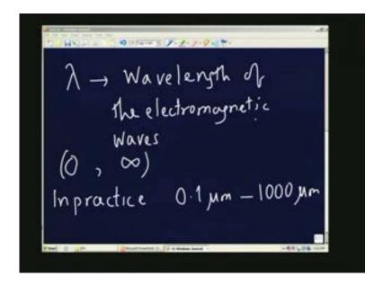
Actually, lambda is the wavelength of what, of the electromagnetic radiation. The power radiated is in the form of electromagnetic waves, the wavelength of the electromagnetic waves, and in principle, it can be from 0 to infinity. This is the interval, but in practice, for the kind of temperatures we are interested in, it will be somewhere between, that is point 1 micrometer to about 1000 micrometers.
