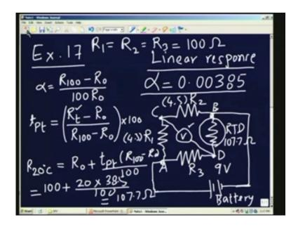
Therefore, by definition of alpha is nothing but  $R_{100}$  minus  $R_0$  divided by 100 times  $R_0$  which is given by point 00385, and we also know that the temperature, according to platinum temperature scale, is given by  $R_t$  minus  $R_0$  divided by  $R_{100}$  minus  $R_0$  multiplied by 100. You have already done this, therefore, I can find out the  $R_t$  at any temperature.
