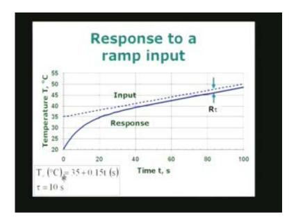
I have taken T infinity which is in degree Celsius. It is given by 35 plus point 15t, where t is in seconds. I have taken the time constant of the sensor as equal to 10 seconds, and I have shown the plot when the temperature of the sensor was 20 degree to start with. So, initially you see that the temperature is increasing and it is trying to catch up with the temperature of the ambient which itself is again increasing and therefore it will never catch up completely.
