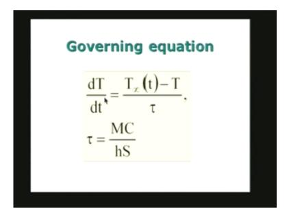
So dT by dt equal to T infinity minus T divided by tau. This is the temperature difference or it is like the voltage potential difference and divided by time constant. Time constant is something like a characteristic time for the particular problem which is given by MC by hS. And in the next slide I am showing the electrical analog of the same situation.
