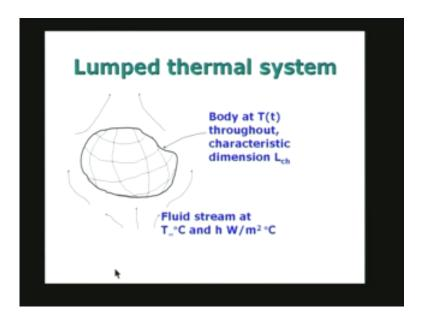
The basic model which we are going to use for describing a temperature sensor is in terms of a lumped thermal system which is schematically shown in the slide here. We have an object. Suppose the sensor is to be represented by this object which is shown here. Of course the shape and size and other things will come later on.
