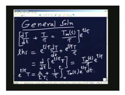
So, general solution to the first order equation, we know that it is dT by dt plus T by tau is equal to T infinity which is a function of time divided by tau. Suppose I multiply throughout by e to the power of T by tau which is an integrating factor. So if I multiply these two, the left hand side becomes e to
