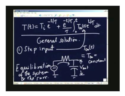
I am going to put T infinity equal to constant. So this will be replaced by constant value T infinity and all I have to do is to obtain this integral and then I will be able to get the solution to the problem. Let us look at that one.
