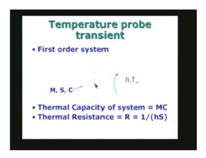
And first for doing that I have given a slightly different schematic here. I have a sensor idealized as a spherical object here. It may be visualized as a spherical shell and I have introduced a thermometer or a temperature sensor somewhere in the shell, and because we are assuming that the shell is entirely at a uniform temperature at any given time, there is no variation of
