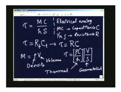
If I look at the electrical analogy or analog MC is like the capacitance, and 1 over hS is like a resistance. And you see that if I show it as capital C and that as R, the time constant for a electrical system is R times C. And exactly that is what we have here. If you want you can show it as 1 over h is the thermal resistance. So I can say it is R thermal and C, MC is actually the C thermal. tau is equal to RC. This is the analogy between the two system that is number one.
