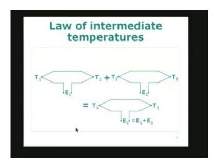
Suppose I have two junctions,  $T_1$  and  $T_2$ , and I measure the electromotive force across the junctions. This is  $E_1$ . I have another arrangement in which the junctions are at temperature  $T_2$  and  $T_3$ , and I measure the voltage for the electromotive forces  $E_2$ . Now, if the junctions are at  $T_1$  and  $T_3$ , here  $T_1$ ,  $T_2$ ,
