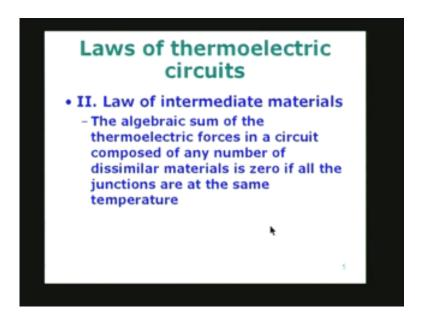
The second law is called law of intermediate materials, which plays a very significant role. As you will see a little while from now, it simply says that the algebraic sum of the thermoelectric forces in a circuit composed of any number of dissimilar materials is 0 if all the junctions are at the same temperature. This is a very important relationship, and we will go back to the thermoelectric circuit and explain it little later, but what does it mean? It means simply this:
