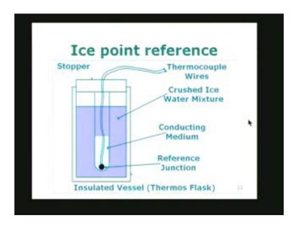
What I have got here is a large vessel. Normally, we use a thermos flask, double walled thermos flask. Inside that I have got a long tube. You can see the long tube here, into which I have put the thermocouple wires, and there is a junction which has formed right here. This black thing is the reference junction and it is immersed in a liquid which is a conducting medium.
