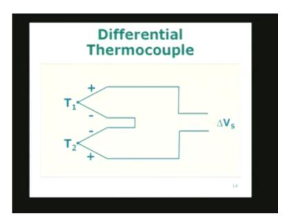
We can also do the following. We can have a differential thermocouple. What is the differential thermocouple? It measures directly the temperature difference between two junctions. Where do we use it? Why do we use it? We will just look at it.
