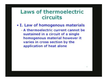
One is, of course, the law of homogenous materials, which simply says that a thermoelectric current cannot be sustained in a circuit of a single material, homogenous material, however, it varies in cross-section by the application of heat alone. Very important. If it is uniform material made of the same homogeneous material, whatever may be the shape, size of the cross-section, and so on, if we simply apply the temperature variation, nothing is going to happen.
