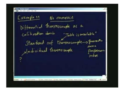
For example; what we will be doing is; for this thermocouple a table is available. The manufacturer has guaranteed that a table is available and you can use the table for this purpose. For this I don't know what it is. Now how do we go about calibrating this individual thermocouple with the help of the standard reference thermocouple. For that what I am going to do is I am going to make a circuit like the following: it is exactly like what we had, the differential thermocouple. This is standard.
