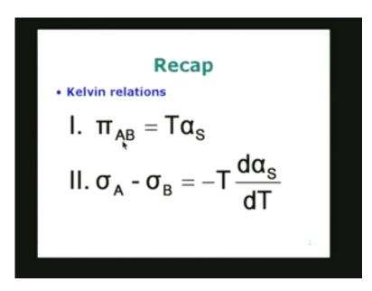
The first one is pi<sub>AB</sub>, the Peltier coefficient or Peltier effect cocoefficient, AB is the pair of materials were chosen, material A and material B is equal to the absolute temperature T times the Seebeck coefficient alpha subscript s. For this is the first Kelvin relation.
