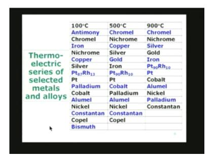
In fact, in practice, what we do is we standardize some thermocouples and we use only those thermocouples, even though in principle any two materials, any two metals, or any two alloys can be joined together to form a thermocouple, it is simply not possible to do that in practice, because it leads to a lot of confusion, and each person will have his own thermocouple, and so on. It is not a very satisfactory state of affairs.
