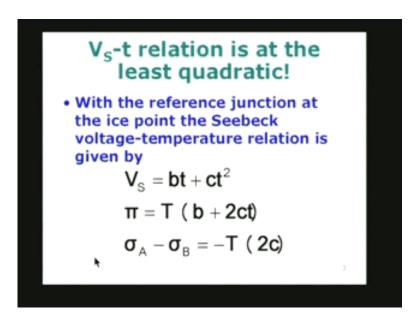
From now onwards I am going to use two different temperatures. Capital T will be representing the Kelvin temperature or the absolute temperature, the Kelvin scale, and I will also use the lower case t for the temperature in degree Celsius. So when ever I use the capital T it is understood that I am referring to the absolute temperature. When I use the lower case t, I am representing, or referring to the Celsius temperature.
