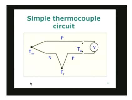
I have the positive wire which I call as P. I got the negative wire and I got the measuring junction that is there. I have made a bead here and the negative material is now brought here. There is a bead with the positive material. So you see that the voltage is measured between the positive and the positive.
