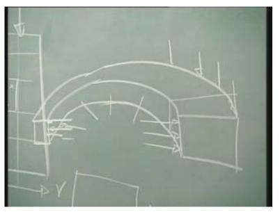
Hence that ring is under automatic equilibrium. You need not specify a boundary condition in the radial direction. In other words, suppose I have a problem where I have this particular tube, a hollow cylinder with internal pressures defined.
