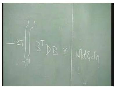
So, you can have 2 pi out and then you have an equation of this form. Now, the only question is r. r is the radius. Where do we get this radius now? r is the radius, where do we get, how do we get this? Remember that we are going to integrate it with respect to or we are going to find out the values at the gauss points and so we are going to get this values at the gauss points and so we need r.
