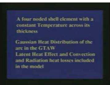
Sometimes it so happens that when the temperatures are large near the welding zone, the radiations also has to be taken into account. But, before that there is what is called as a Gaussian heat distribution for the welding process that has been put. In other words, when you weld you give a heat input.
