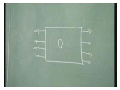
Let us say that I take a sheet like this, put a hole in the centre and I want to pull this. As you know, I have to give a boundary condition; I cannot just pull it like this. So, I do it by two means. One is by fixing this side, the left hand side I am going to fix.
