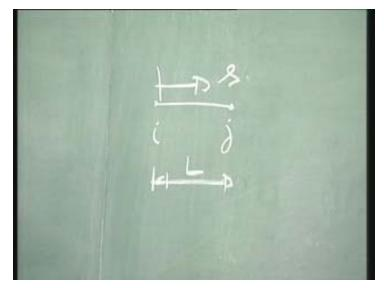
Let us say that the length of this element is equal to L. Now, I am going to put a local coordinate system to it. Let me put a local coordinate system, such that it is depicted by s. What does it mean? s is equal to zero at i and s is equal to L at j. Is that clear?
