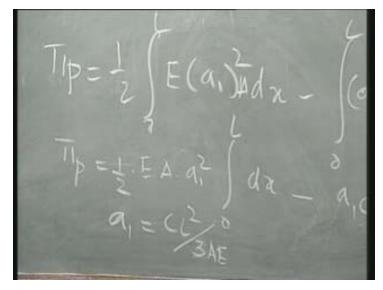
So, this is equal to, u is equal to  $a_1x$ . So, du by dx will give me epsilon x and that is equal to  $a_1$  and that is equal to this expression. So, CL squared by 3AE gives me the, what is that it gives? Strain multiplied by E gives me the stress. So, what does it mean? It means that, now the stress, if I have taken, when I have taken the one term, is constant throughout the bar, which is definitely rather an approximation.
