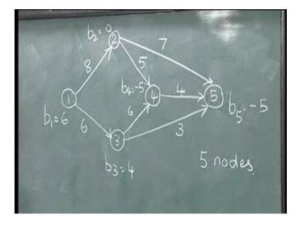
The minimum cost flow problem is now described using this numerical example. We consider the network that has five nodes and it has all these arcs as described in this figure. Each of these arcs has an arch weight which represents the cost of transportation or cost of flow associated with this arc. For example, it costs 8 to transport a unit from 1 to 2, while it costs 6 to transport from 1 to 3. In addition, we also have some values associated with these nodes.
