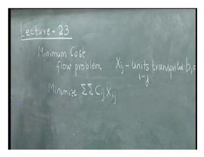
The minimum cost flow problem will have a primal, which is minimize double sigma  $C_{ij} X_{ij}$ , where  $X_{ij}$  is the units transported from i to j,  $C_{ij} X_{ij}$  is the total cost of transportation.
