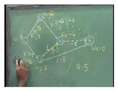
I have 1 2 3 4 5 nodes, have a solution X equal to 5, X equal to 1, X equal to 5, and X equal to 5. This is the solution. We again fix  $w_5$  equal to zero. We get  $w_3$  from  $w_i$  minus  $w_j$  equal to  $C_{ij}$ .  $C_{ij}$  is 3, so you get  $w_3$  equal to 3. From here,  $w_i$  minus  $w_j$  is equal to  $C_{ij}$ .  $C_{ij}$  is 6, so you get  $w_1$  is equal to 9, 9 minus 3 equal to 6.
