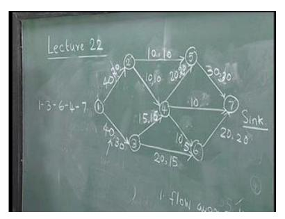
1 to 3 is a forward arc, there is an arc from 1 to 3; 3 to 6 is a forward arc, there is an arc from 3 to 6. 6 to 4, there is no arc in this network 6 to 4, but we are still considering it because there is an arc from 4 to 6. Then, 4 to 7 is a forward arc with an arc going from 4 to 7. Let us consider this once again. Now, 1 3 is a forward arc, because there is an arc from 1 to 3, 3 6 is a forward arc, 6 to 4 is a backward arc and 4 to 7 is a forward arc.
