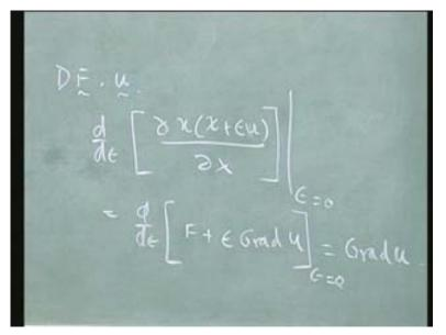
How do I do the linearized part of the deformation gradient tensor or in other words, what is the D F dot say, u? How do I do that at a particular configuration chi. This is given by d by d epsilon of dow of epsilon v at a particular configuration dow X at epsilon is equal to zero, which can be written as d by d epsilon with respect to small chi or small x, we can do that; so, F plus epsilon into Grad sorry, not v, u, Grad u at epsilon is equal to zero, which gives me Grad u.
