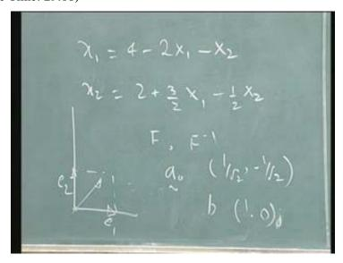
For a two dimensional problem, the deformation for a two dimensional problem, the deformation is given by the explicit equation  $x_1$  is equal to 4 minus  $2X_1$  minus  $X_2$  and small  $x_2$  is equal to 2 plus 3 by 2  $X_1$  minus half  $X_2$ . Now, determine the matrix
