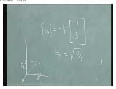
So, that is what I would call as say,  $b_0$  is equal to minus 1 by 5 1 and 3 and what is the length of that? The length of  $b_0$  is equal to 2 by 5, root of 2 by 5. In other words, what it means is that a line element which is now currently of unit length was in fact root of
