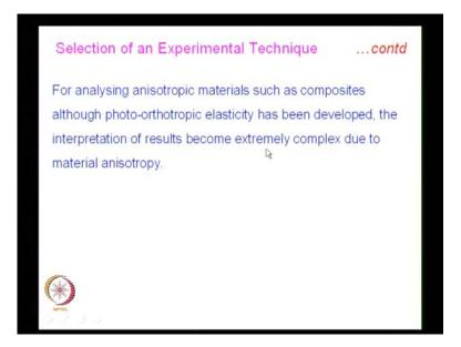
For analyzing anisotropic materials such as composites, although photo orthotropic elasticity has been developed the interpretation of results, become extremely complex due to material an isotropy.
