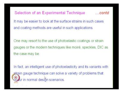
It may be easier to look at the surface strain in such cases, and coating methods are useful in such applications. One may resort to the use of photo elastic coatings or strain gauges or the modern techniques like Moire, speckles, digital image correlation as the case may be. In fact, an intelligent use of photo elasticity, and it is variants with strain gauge technique can solve a variety of problems that occur in normal design scenarios.
