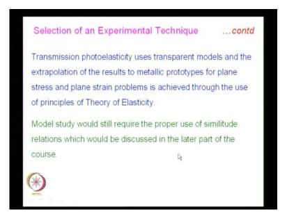
Transmission photo elasticity uses transparent models, and the extrapolation of the results to metallic prototypes for plane stress, and plane strain problems is achieved through the use of principles of theory of elasticity. Your actually using a model, and model study would still require, the proper use of similitude relations which would be discussed in the later part of the course.
