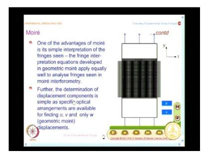
And other concept, which I wanted to say, was that you are able to get the displacement information, comfortably separated in moiré analysis. And purposely this is taken like this, I have a specimen with a cross grating, but I view this specimen with the horizontal grating. So, what is the displacement I get, we have already seen, once you have horizontal grating, what is the displacement you get; you get the displacement perpendicular to that.
