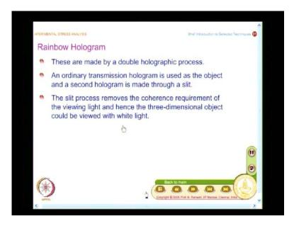
And what you have here is these are made by a double holographic process. An ordinary transmission holograms is used as the object; and a second gram is made through a slit it, is an optical requirement and the focus here is, I want to see the reconstruction, without going into complicated optics, just normal white light should be good enough that is the purpose behind it.
