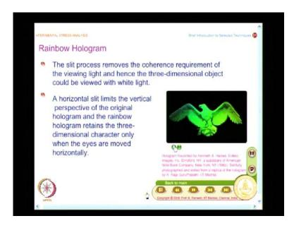
So, what you have here is the slit process, removes the coherence requirement of the viewing light and hence the three-dimensional object, could be viewed with white light.
