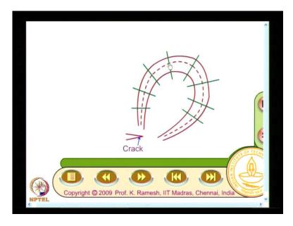
Suppose, I have a complex fringe pattern like this, which you see at the tip of a crack the fringes are very sharp near the tip of the crack and they are very broad here. I cannot take
