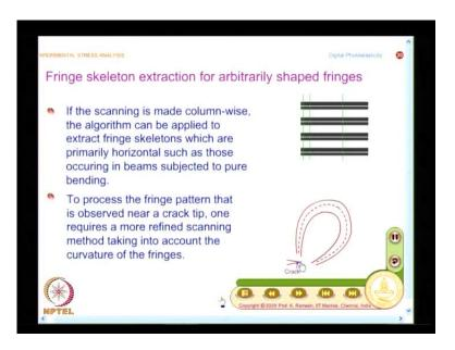
And what we saw was in the global methods, we took two simple examples, one is vertical fringes and horizontal fringes. Suppose, I have horizontal fringes like in a beam, I can develop a scanning methodology which is perpendicular to the fringe areas, it will automatically pick out the minimum intensity, so when we join them you will get a fringe skeleton.
