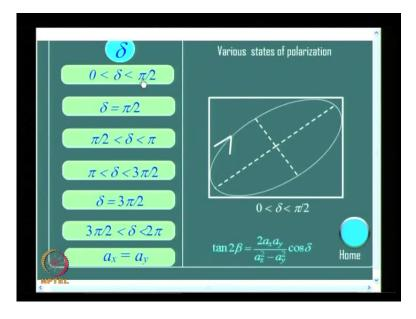
So, when delta changes, you can easily see that beta also changes. In addition what you find is, when I have delta for different ranges 0 to pi by 2 or delta equal to pi by 2, pi by 2 between pi by 2 and pi, what you find is, then you go and actually plot the tracer of the light ellipse. You find the rotation is different and that is what is illustrated in the series of graphs.
