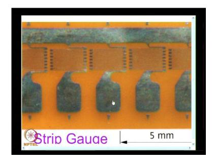
So, in order to simplify for such applications you also have what are known as strip gauges that is what is shown here, I think I will enlarge it and then show you what is the strip gauge. So, what you have here is you have strain gauges pre aligned available in one backing very small strain gauge and even to solder and connect and paste, all these are very complex issues, but the advantage is you are able to get strain at short distances very comfortably.
