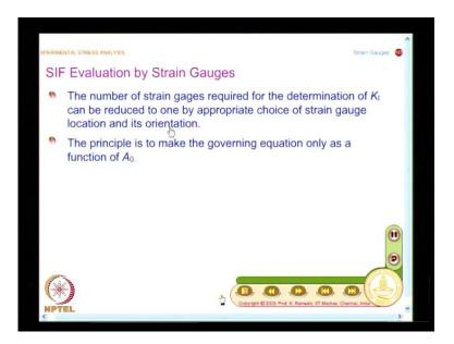
So, the idea here is the number of strain gauges required for the determination of K1 can be reduced to 1, by appropriate choice of strain gauge location and its orientation. See essentially my interest is to knock of B 0 and A 1. So, I want to knock of B 0 and A 1 terms.
