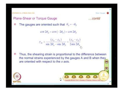
So, you will have only 1 term in the expression for gamma x y. So, when I have theta A equal to minus theta B I get gamma x y as Epsilon A minus Epsilon B, divided by 2 sin 2 theta A. And you know in normal strain gauge measurements you connect 1 strain gauge
