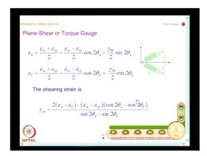
Where you see one layer after the other, you know now we move on to an interesting class of special gauges. First we take up a plane shear or torque gauge and what we are going to do here is we are going to look at a very generic arrangement and in this you have two strain gauge.
