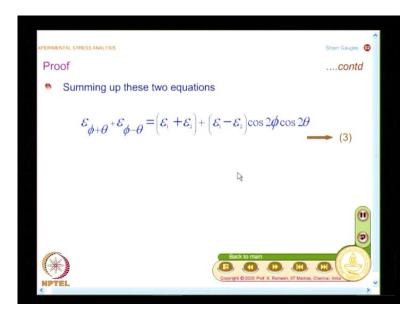
So, we will develop a complicated gauge pattern to start with, in an unknown situation you will do this, but you will also find out whether you could use a simple normal strain gauge for stress measurement and when I add these 2 strain quantities I get this as Epsilon 1 plus Epsilon 2 Plus, Epsilon1 minus Epsilon 2, multiplied by cos 2 pi into cos 2 theta and I will further simplify my focus is finally to get the addition of these 2 strains
