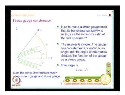
And there is a subtle difference between what we saw as a torque gauge and what we say as a configuration for the stress gauge here also I have 2 elements orientated at plus theta and minus theta, but what the subtle difference is these 2 elements are join they are not independent elements.
