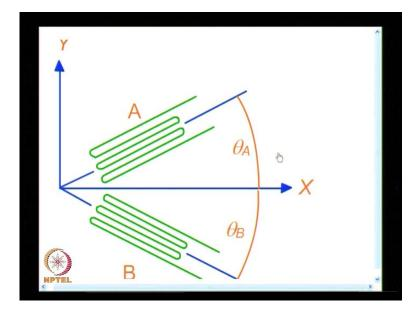
Elements which are oriented at angles theta A and theta B, and you have the reference axis as X and Y. So, you have 1 strain Gauge element measuring strain a long theta equal to theta A and another strain gauge element which is measuring strain along theta equal
