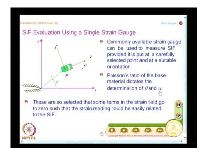
So, what I am going to do is I want use the common strain gauges, so I will have the orientation theta, but at orientation theta I will have the strain gauge align that angle alpha. So, for this value only I would find out the strain along this direction and now question is how to select the theta and alpha? That is what you will look at it, you make a needs sketch of this diagram that illustrates how to use a single strain.
