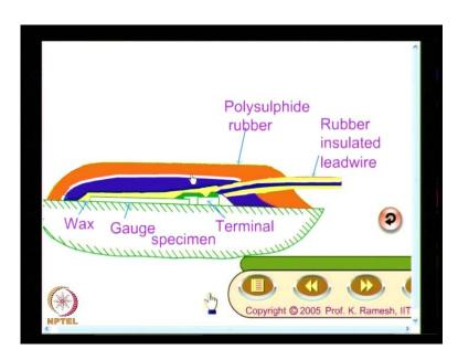
So, what you essentially have is on the specimen you have the gauge, then you have a coat of wax, then you have a coat of rubber, then you have a aluminum foil and have a final coat of polysulphide rubber and this is also you can see it as animation.
