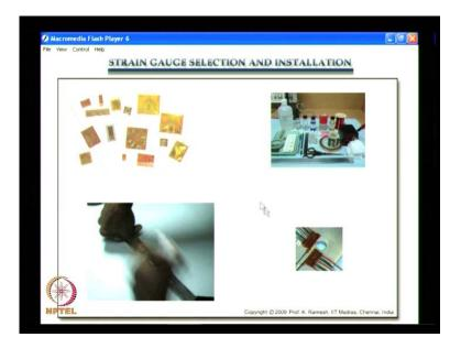
Instrumentation, strain gauge selection and installation is very crucial, we saw that variety of patterns exit and there is a very elaborate kit available. And there is a procedure how to apply the bonding and a simple signoculte cement gets cured by a thump pressure, that is what is illustrated here. And you press it with a gauges panks and put it with a thump pressure and after about 2 minutes the bonding is completed and this shows use of strip gauges and finally.
