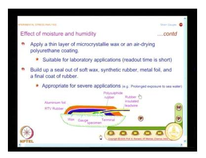
So, when you learn that it has to be protected against moisture, one of the simpler approaches is apply a thin layer of microcrystallie wax or an air drying polyurethane coating and this is good enough for laboratory measurements and your read out time is essentially short. On the other hand if we have to make strain measurements under
