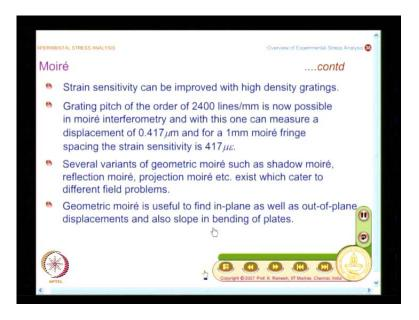
So what you find here is, strain sensitivity can be improved with high density gratings, and what you find is 2400 lines per millimeter is now possible. It is the theoretical limit; people have achieved the theoretical limit by real hard work. And with such high density
