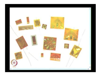
So it is a very versatile technique, it is very widely used and as I also caution earlier it has be used with care. And what you see here is you have a array of strain gauges for various applications and this you have a hole so this is meant for residual stress component. And I mention strip gauges this is what a strip gauges you have a series of strain gauges available in a strip and likewise you have varies grid configuration available.
