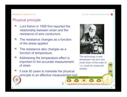
This is on various manufacturers you have given this and what is the physical principle this technique is based on. And it was reported way back in 1856, it was reported by Lord Kelvin and he found out a relationship between strain and the resistance of wire conductors.
