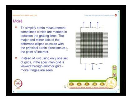
And now what I am want to do is people fell that, of just using a one grid, if I have more than one grid it makes it little more comfortable that is how moiré started developing. And what you find here is I have a specimen, on the specimen I have a grid and I view it through another grid like this. And what you find here is I have stretched it slightly, but I see a play of fringes on the specimen I am able to see the fringes they are horizontal fringes.
