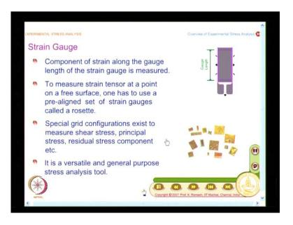
My focus is only to bring out what is the basic physical information each of the techniques is based upon and we will go from the technique like strain gauges to start with, because this is the most widely used technique. And as I mentioned earlier in this you get component of strain along the gauge length of the strain gauge is measured and here you have the typical enlarged view of the strain gauge and you call this as the gauge length.
