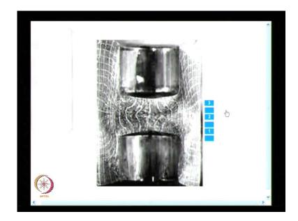
And what you have here is in the case of metal forming processes what they have is they have a billet and they will put a grid. You can see the grid here these are known as grid methods and what I have is when I do the metal forming operation I do a large plastic deformation.
