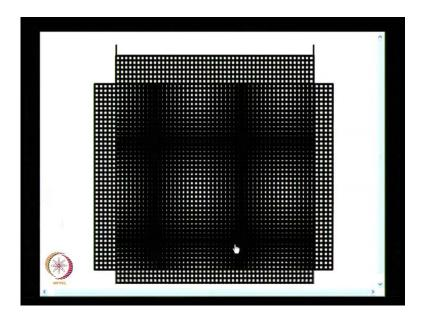
So if I have a finer grating, I have a better chance of measuring small deformation. And what you have here is I have two grids, I have this I called as master grating. This attached to the specimen which is pulled, because of poison ratio effect the thickness comes down, and you see horizontal you see horizontal fringes as well as vertical fringes.
