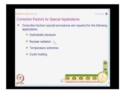
Here, the topic itself says that what are the correction factors for special applications? You know you cannot be doing strain gauge only for simple applications you need to work and find out what happens inside a pressure vessel because you all known from Lami's problem, the inner surface of the pressure vessel is subjected to maximum amount of tensile stress. So, there are occasions where you need to find out what are the strain develop in the inner surface?
