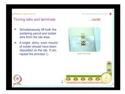
So, what is the recommendation? The recommendation is lift the soldering pencil and the solder wire from the tab area simultaneously. And if you do this, what you get? A bright shiny even mound of solder should have been deposited on the tab if not, repeat the process. And you have a nice example you know you saw the counter example earlier and now you see how nicely the solder deposit is done at the four points. In order to get this you need to follow a sequence and respect the recommendations.
