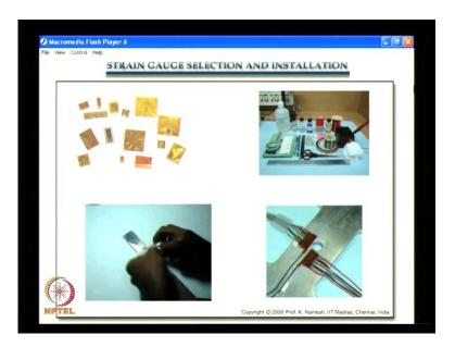
And when you go for strain gauge selection and installation, you have various patterns available and for a plate with the hole you have a strip gauge that is pasted here. And this shows what are the accessories that you require for strain gauge bonding and this gives
