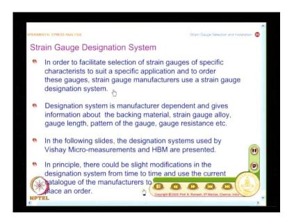
So, it does two jobs one is to facilitate selection of strain gauges of specific characteristics and also to order these gauges and obviously, the designation system is manufacturer dependent and gives information about the backing material, strain gauge
