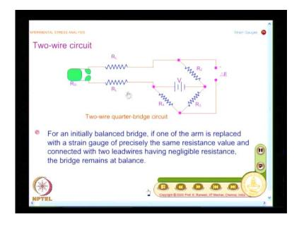
And suppose somebody gives you a strain gauge, what will you do. You just connect the strain gauge to the wheat stone bridge. I have two points, and I take a wire and then connect it to the whichever arm that I want to do it. I connect it appropriately and that is how you would normally connect a strain gauge - by connecting two wires. What is a influence of the lead wire?
