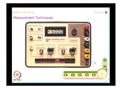
Now we go and look at what are the measurement techniques. I am showing a typical strain gauge meter and I would like you to draw your attention to few finer aspects. First issue is, if you look at very carefully, this is for 120 ohms, this is for 350 ohms; it may not be clear on the screen, but you know there are provisions available for selecting internal resistors of 120 ohms or 350 ohms.
