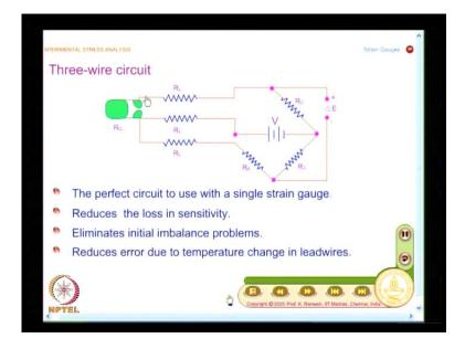
The via media to overcome this is a three wire circuit. I want you to make a decent sketch of it and instead of two wires coming from the strain gauge, from one of the (()), I take two wires and intelligently connect them to the wheat stone bridge. This portion does not change, but how do you connect the strain gauge to the strain meter in forming the bridge is slightly modified and shown here.
