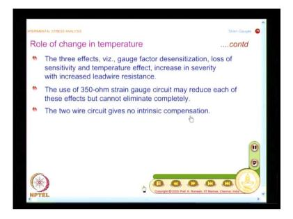
So, what you find is, the gauge factor desensitization or loss of sensitivity and temperature effect increase in severity with increased lead wire resistance. So you have to account for it in practical applications. So one way of looking at this is, go in for a 350 ohm strain gauge. This can reduce each of these effects, but cannot eliminate any one of them completely.
