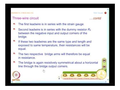
And whatever I have said earlier is summarized as points: the first lead wire is in series with the strain gauge, the second lead wire is in series with the dummy resistor R 4 between the negative input and output corners of the bridge; so I have lead wire on two different arms.
