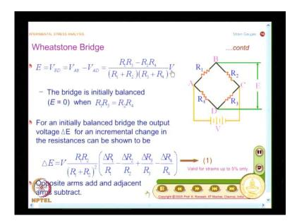
Our focus is, what happens when the resistance changes slightly and whenever I do any instrumentation, I initially balance the bridge and while balancing the bridge, I essentially make E equal to 0, that is, V B D equal to 0 that gives be an expression V B D as R 1 R 3 minus R 2 R 4 divided by R 1 plus R 2 into R 3 plus R 4 into V; when I make equal to 0, this gives me a condition R 1 R 3 should be equal to R 2 R 4. So, when I construct Wheatstone bridge, I need to maintain this relationship.
