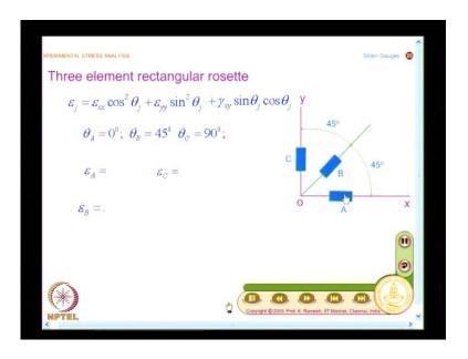
And let us see two famous configurations of the rosettes. And one of the rosette is called a rectangular rosette is primarily because I have a strain gauge along the X axis and the second strain gauge at 45 degrees and the third strain gauge is along the Y axis. So, what is the strain measured by the strain gauge A? If I have this as my reference axis, I could simply say its equivalent to epsilon X and strain measured by the strain gauge C is epsilon Y.
