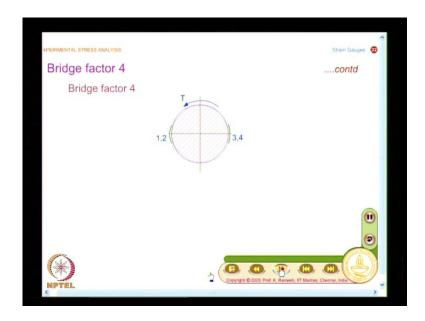
And you know, I am going to give you one more example which I leave it as a home exercise. You know, I have taken a shaft under torsion and what I want you to do is, I want you to identify how do I paste the strain gauge 1 and 2, how do I paste the strain gauge 3 and 4, and how do I connect them into Wheatstone bridge for me to measure the torque.
