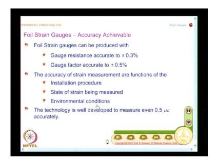
See, what I have been mentioning is, strain gauge instrumentation, we are looking for measuring small quantities. So, we have to pay attention for every minute detail. We looked at strain sensitivity of a conductor, then we graduated and looked at strain sensitivity of grid, and then, we also looked at bridge sensitivity in bridge sensitivity.
