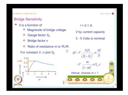
So, I have the bridge sensitivity, it is the function of magnitude of bridge voltage, gauge factor S g, bridge factor n and the ratio of resistance R 2 by R 1. See, what we want to look at is, your initial balance only gave me a condition between the resistances; now I will find out for maximum sensitivity what should be the value of the ratio R 2 by R 1. And we write this expression delta E in a much convenient fashion, I have this as V into
