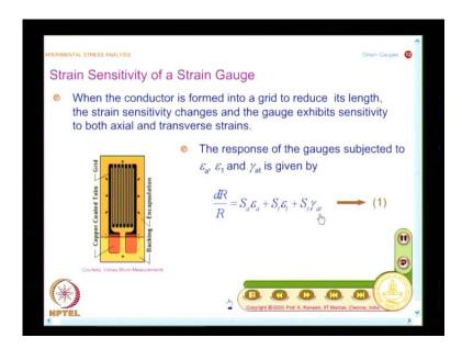
So, now, we look at what is the strain sensitivity of a strain gauge. Because we have looked at, the conductor is formed into a grid to reduce its length, the strain sensitivity changes. Because it is now made into a grid, the gauge exhibits sensitivity to both axial and transverse strains.
