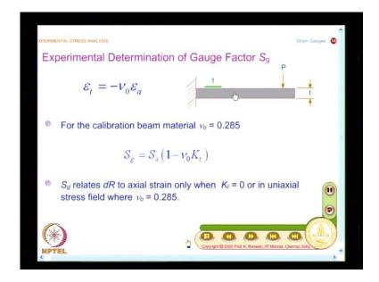
Because I have been saying, Poisson's ratio has a role to play in all the experimental technique and what does the manufacturer do? He takes a cantilever, puts the strain gauge and for a given load or a set of loads, he would find out the strain from the analytical solutions, he would be able to correlate and establish the parameters. When you do an experiment like this, Poisson ratio of the calibration material comes into plane.
