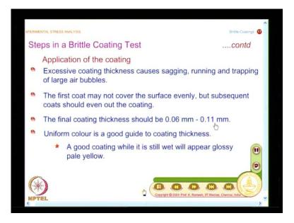
And how do I access, I have reached the final thickness? You know, color is very important; you know human brain is very sensitive to observing the color. So, if I have a uniform color, it is a good guide to coating thickness.
