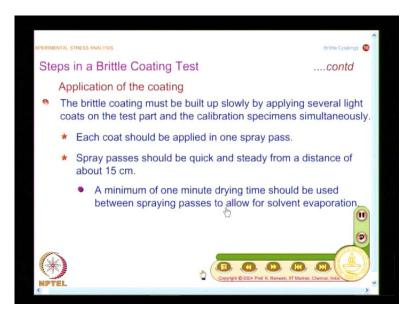
And after undercoat, now you get on to application of the coating and how do you apply the coating? You have to build up the brittle coating slowly by applying several light coats on the test part and the calibration specimens simultaneously.
