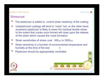
And you should also keep in mind, strain sensitivity is a function of environmental temperature and humidity at the time of the test, which we have also seen when we are talking about the calibration and plasticizer should be appropriately controlled.
