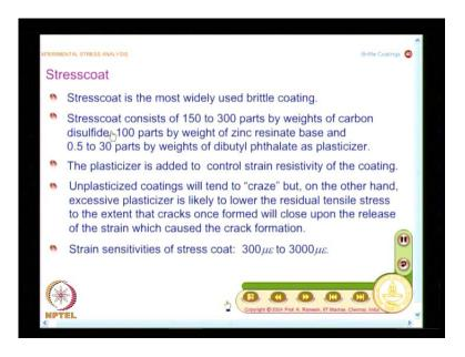
What is the type of coating that is available now? You have what is known as stress coat. I said that initial coatings were naturally formed coatings, then we saw the first coating was a mixture of (()) and alcohol and what you have widely now is called stress coat. Stress coat consists of 150 to 300 parts by weights of carbon disulfide, 100 parts by weight of zinc resinate base and 0.5 to 30 parts by weights of dibutyl phthalate as plasticizer.
