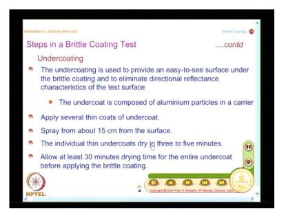
The third step is to provide an undercoat and what is the use of this undercoat? Undercoating is used to provide an easy- to- see surface under the brittle coating and to eliminate directional reflectance characteristics the test surface; it is very important, because you have to go and identify the cracks and you must have a convenient detecting the cracks.
