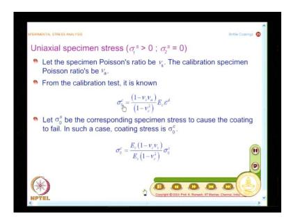
Now, I have an actual prototype also fails only with one specimen stress acting on it, the other specimen stress is 0. Now, let us look at how the interpretation can be done. And we have done a calibration test, from the calibration test what we have found out? We have find out the failure stress of the coating.
