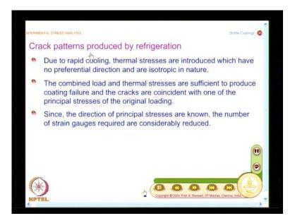
The general level of stress increase that is what you have. Due to rapid cooling, thermal stresses are introduced which have no preferential direction and are isotropic in nature. And what you have is, the combined load and thermal stresses are sufficient to produce coating failure.
