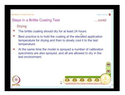
And the final process is how you do the drying. And you should note that brittle coating takes 24 hours for drying it is not immediate; whereas the undercoat took about half an hour, whereas the actual coating, you must allow 24 hours.
