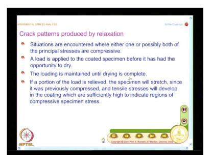
What you do is, when I go for compressive stresses which is known as crack patterns produced by relaxation, you load the specimen first; a load is applied to the coated specimen before it has had the opportunity to dry; the loading is maintained until drying is complete.
