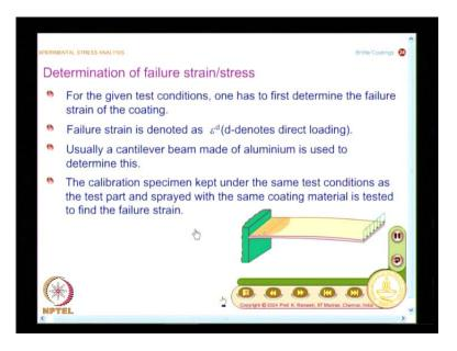
And what is the first step in the case of brittle coating? See, we have all along looking at in any of the experimental techniques, you have to find out what is known as calibration constant. In transmission photo-elasticity, you had sigma as the calibration constant that you need to find out; in photoelastic coating, you need to find out k.
