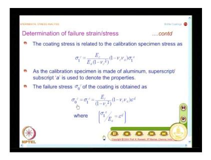
And from whatever the expression that you have seen earlier, it is possible for you to write an expression for coating stress sigma 1 c and I am having only a uniaxial specimen stress; the same coating stress expression have two terms, one with sigma 1 x and sigma 2 x; since I am using aluminium as the calibration specimen, instead of using s as your sub script or super script I use a.
