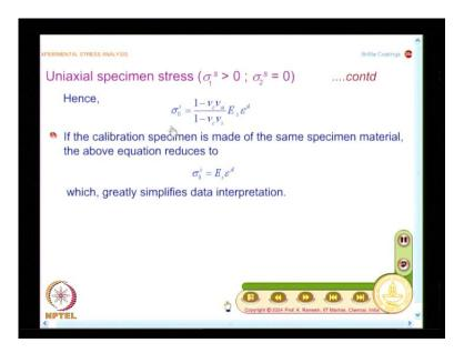
Now, I can bring in; I can express sigma naught x and a different way, where I will find out that if I use a specimen for calibration same as the actual prototype material, then my problem is less and that is what is shown in the slide.
