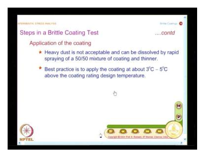
So, when you face a problem, you also have a solution. Heavy dust is not acceptable and you can dissolve it by rapid spraying of a 50 by 50 mixture of coating and thinner; so, this is the beauty. When you look at the procedure, you know, the manufacture has looked at all aspects of applying the coating, because in all coating techniques only the coating is properly formed, data interpretation is meaningful; this you cannot ignore it.
