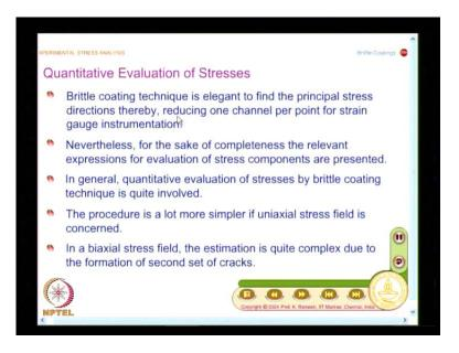
Now, let us look at how I do quantitative evaluation of stresses and this is what I emphasis again and again. Brittle coating technique is elegant to find the principal stress direction thereby, reducing one channel per point for strain gauge instrumentation.
