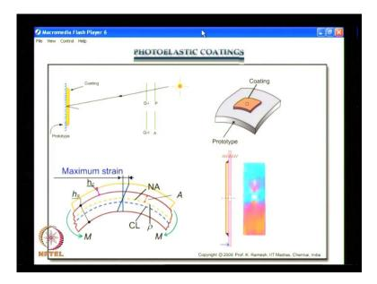
In summary what you can look at is, you have a simple optical arrangement, and then I said for all coating techniques. The coating has to be bounded very carefully on the prototype and we also assume that strains are faithfully transferred from the prototype to
