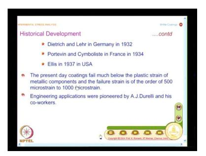
That is what you have to look at? It is started with identifying zones of plasticity in model and failure strain is of the order of 500 to 1000 micro strains even less now, people say even 3000 micro strain is possible. So, you have material research contributed to development of better coating materials, which have more sensitivity for failure here the coating has to fail.
