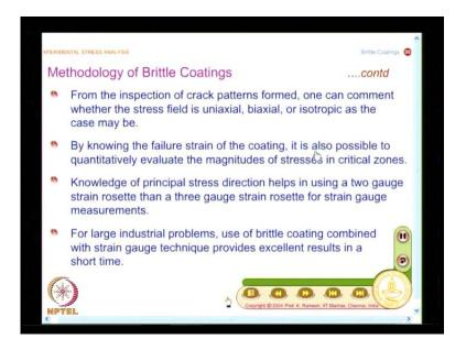
And what is the important is like in optical techniques; here also I see whole field information by looking at the crack patterns formed one can comment whether the stress field is uniaxial, biaxial or isotropic. In fact, in some of the earlier studies even to identify zones of uniaxial, biaxial and then isotopic was an issue, it was large problems. Suppose, I know in a particular region I have only uniaxial state of stress, then I can reduced a strain gauge channel that is the advantage.
