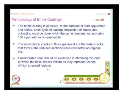
And another aspect, which will have to keep in mind, is the brittle coating is sensitive to the duration of load application. So, you have to have a particular cycle to follow for each cycle of loading, inspection of cracks and unloading must be done within the same time interval and this varies depending on the coatings, it probably something like hundred second per interval is reasonable people also code five minutes.
