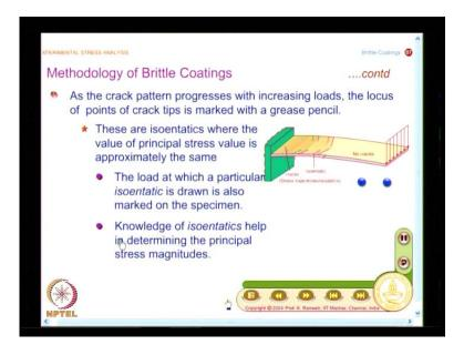
And what you have is, the crack pattern progresses with increasing loads, the locus of points of crack tips is marked with a grease pencil. We will see that this example and what you have here is, I have a cantilever beam, which is subjected to end load and if
