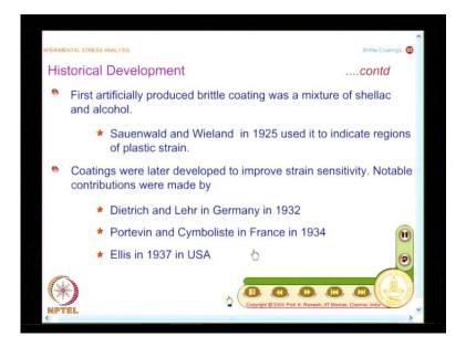
And it is desirable look at what are the contributions by various scientists? And it is also interesting to see, what was the first artificially produced brittle coating? We had seen naturally formed coatings earlier. The first artificially produced brittle coating was a mixture of shellac and alcohol and this was used by sauenwald and wieland in 1925 to indicate regions of plastic strain.
