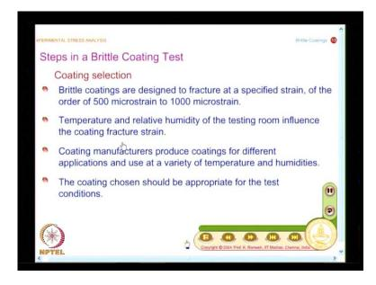
And you know once you come to a brittle coating test, the first step that you need to do is you have to select a coating and if you look at any brittle coating test any supplier whose supplies coating, he gives a different set of coatings for a variety of temperature and humidities.
