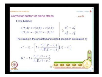
When I go to the force balance, I can write sigma 1 u H s into d y, because this is the area and this could be a... there could be a force component from the coating, there could be a force component to specimen and you will have the expression written down like this sigma 1 s into h s into d y plus sigma 1 c into h c into d y known similar fashion I can also find out what is the force on the other direction and I get this as.
