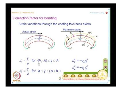
Now will move and find out how do I go about for a correction factor when the specimen is subjected to bending. So, what what you have here is if I have a specimen which is
