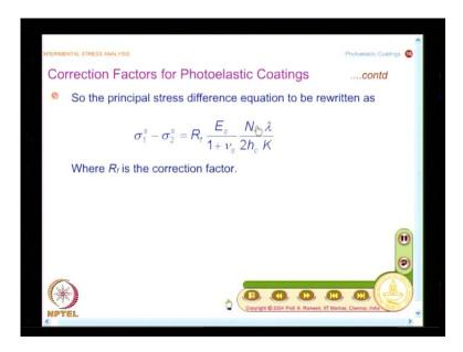
And we will take a one of the very simple problems to start with and before, we are going to that as I said the final expression that you need to know in reflection photoelasticity is as follows. A difference in principle stresses of the specimen namely sigma 1 s minus sigma 2 s is given as R f into young's modules of the specimen divided by 1 plus nu s into N by 2 h c lambda by K and whatever the discussion we had on color code is equally applicable in reflection photoelasticity.
