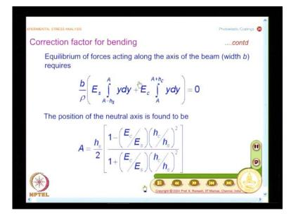
And first let me write the force balance. So, the force balance you could write it in this fashion straight forward on a beam and pure bending the net force is zero for I have 1
