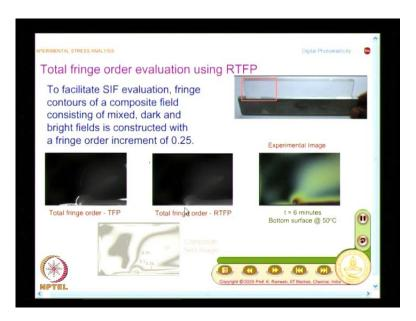
And the total fringe order from TFP is like this, which is improved by RTFP, and finally from this, you have the fringe patterns extracted from the whole field, and you find there is lot of data near the crack tip.
