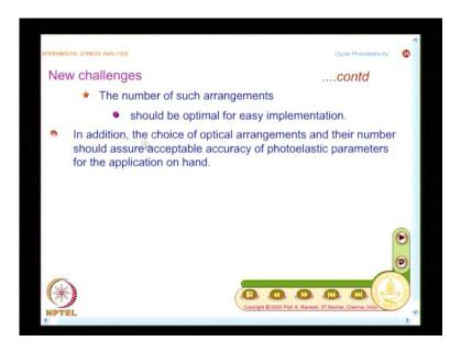
Now, what you have is methods, which uses conventional polar scope also and you also have when you looked at the optical arrangements how many number we have to use? How many parameters that you have? I have to find out the isochromatic parameter isoclinic parameter and the background light intensity. So, three should be good enough, then people found 4 is necessary from accuracy point of view you have to go for the more and more methods.
