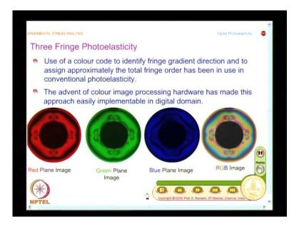
Now, we will take it up what is three fringe photoelasticity, and we have seen in conventional photo elasticity. The color code is use to identify the fringe gradient direction and also to assign the total fringe order approximately, this has been the focus in conventional photo elasticity with the advent of color image processing hardware this approach is easily implementable in digital domain.
