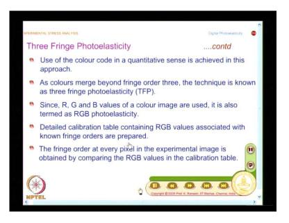
The methodology is as follows. So, you aim at use of the color code in a quantitative sense that is a focus. We have looked at color code more from identifying the fringe gradient direction with the digital hardware. It is possible to get the fringe orders in a quantitative manner with the color code.
