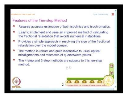
So, the first achievement is it assures accurate estimation of both isoclinics and isochromatics. The methodologies easy to implement and uses an improved method of calculating the fractional retardation that avoids numerical stabilities. In fact, this was a very difficult problem many researchers have looked at it and finally, we have a methodology, it is not? So, simple.
