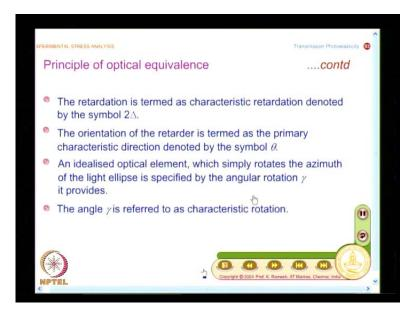
And analyze it by Jones calculus and whatever I have said, the retardation is termed as characteristic retardation labeled as 2 delta. The orientation of the retarder is termed as the primary characteristic direction denoted by the symbol theta. The rotation is given by gamma; the gamma is given as labeled as characteristic rotation. So, these are all the three quantities determined experimentally for a three-dimensional photoelastic analysis.
