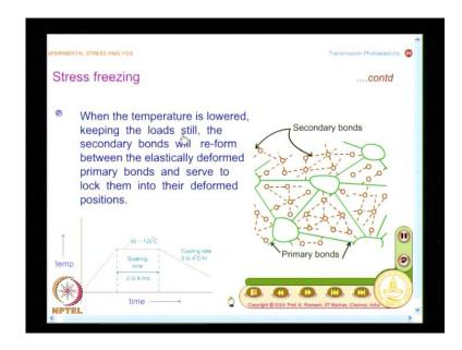
And this is what you have thermal cycling process, very similar to what I do in the case of keeping a string compressed, when the temperature is lowered, keeping the loads still, and the secondary bonds will re-form and prevent the elastically deformed primary bonds to come back it is original position. And hence, the stresses are lock, and at the end of the process I remove the load.
