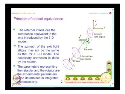
I have an incident light ellipse. So, it gets transformed whatever the transformation by the retarder may not guarantee the same azimuth, and rotator rotates it is... So, that the azimuth matches with the actual three-dimensional model. So, whatever the three-dimensional model you had and we are only confining to the particular light path. Whatever at happens that light path is replaced by a rotator a rotator here and a retarder.
