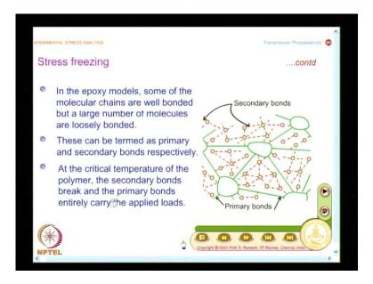
And what you have here, I have this epoxy can be thought of as assembly of secondary bonds as well as primary bonds. When I have an epoxy schematically this is shown, in epoxy models some of the chains are well bonded, but a large number of molecules are loosely bonded. So, the well bonded bonds you call it as primary bonds and the chains that are loosely bonded you call them as secondary bonds.
