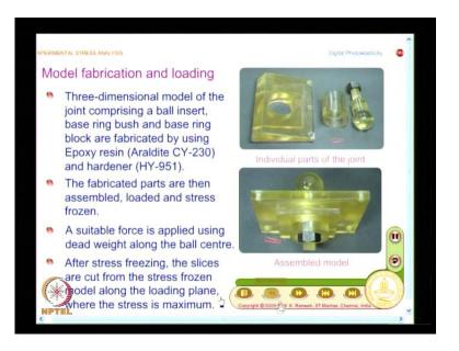
And also show you another example, which is a much complex problem. This is just to give a flavor, what kind of complex geometric shapes people have made, and this is a model that is used in a rocket to transfer that thrust from a stress motors to the main body, and you have a ball and socket joined here. So, I have a spherical ball here, and you have a threaded connection, you have a bush and the relative size is shown with the help of a figure of jump clip here.
