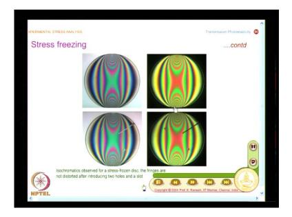
And here you have the fringe patterns, I have a bright field as well as dark field and this is the fringe pattern that you get after the thermal cycling process and what you see here I will also enlarge it, what you see here is after the thermal cycling processes. A flat is made which is very clearly seen in a bright field, and you could see very clearly. There is no discontinuity in this stress distribution it only that this portion is removed.
