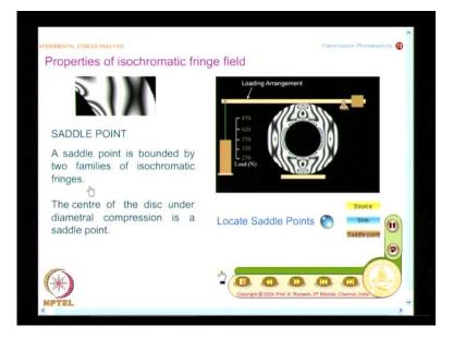
And what you find here is, I have four points in an inner boundary 1 2 3 4, and four points on the outer boundary 1 2 3 4, where the fringe order is 0, and fringe order is also 0 at these two points. Whenever I cross the fringe order 0, the sign of the boundary stresses changes on the boundary, you have to understand that. When I cross 0, I can cross only when there is a sign change and you have two strings in the ring under diametral compression.
