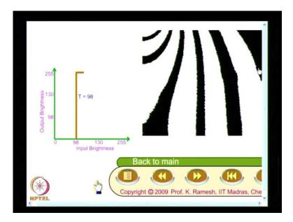
And if I change the threshold optimally, suppose, I make it as 98 which is the very good threshold for this problem, I see so many fringe contours beautifully demarcated. This is one of the greatest advantage in photo elasticity, even a simple thresholding operation you are in a position to identify fringe areas. Because, if I want to do a binary based
