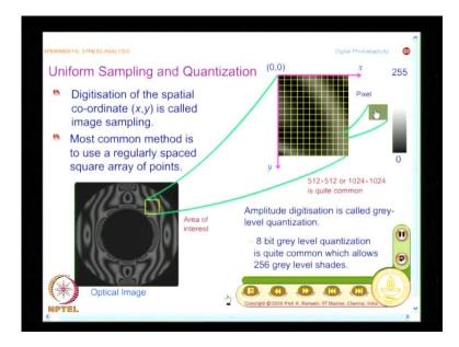
So, you identify the image as an assembly of small pixel elements, and for each of this pixel you assign a number between 0 to 255. If you are processing a negative, it will give the light transmitted, and if you are processing a positive, it will give the light reflected. So, at the end what you get is, by using a digital camera, you are able to get intensity data at video rates, that is the advantage.
