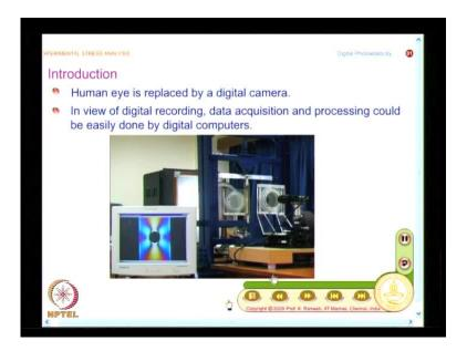
And what we introduced was in the case of digital photo elasticity, you replace the human eye by an electronic eye, you have a digital camera, these are essentially charge coupled devices, you call them as CCD camera. And once you use a CCD camera, it is possible for you to get the image as an assembly of numbers, and this is essentially called sampling and quantization. First, you do a spatial discretization, that you call that are
