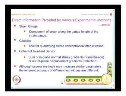
See most of the optical techniques are non contact, if you look at the optical techniques there all non contact techniques. Now I am showing a strain gauges when you go to strain gauge what you do? You actually take a strain gauge paste it on the specimen.
