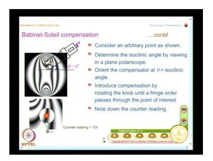
Now, we go back and then see how do I use this information. So, we have determined the isoclinic angle by viewing in a plane polariscope, and what I mean to do is orient the compensator at theta equal to isoclinic angle, so that is what you see here.
