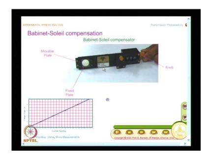
So, what we will do is we look at Babinet-Solell compensator, as well as compensation by using the analyzer. And you have readymade equipment's available for Babinet-Solell compensation. And you can see here, I have a window and I have another plate that is coming out, so I have a fixed plate, and I have another plate which moves and you can also see that there is a counter. So, this is the commercially available Babinet-Solell compensator, this is from a (()) measurements group.
