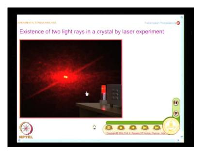
And in order to give you an idea, it is indeed so, we have also rotated a crystal and we saw that one dot becomes two dot, which indicates that the incident light in relation to the optic axis has a role to play. So, now the stage is set for how to analyze this mathematically.
