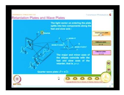
So, what this shows is, I have a source of light, I have a plane polarizer, after the plane polarizer, I have a plane polarized light, hits the crystal plate. As soon as it touches the front surface, it splits into two components. Because within the crystal you will have two refracted beams, you are not going to have only one refracted ray. And these two refracted rays will have different amplitude, which are shown, which is depicted by the angle theta.
